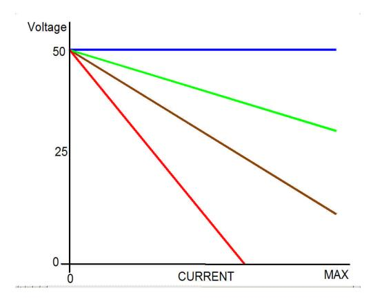
The above graph shows how the current control works. The voltage control is set at 50 volts. When set to the maximum (full clockwise), the voltage will stay at 50 volts (blue line) and is constant voltage. As the current control is rotated counterclockwise, the slope is increased. The red line is with the control fully clockwise.
