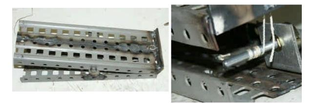
TIG can be done the same as arc welding. A torch with a gas valve can be used with scratch start. For better control and waste less gas, a remote footpedal can be used.
