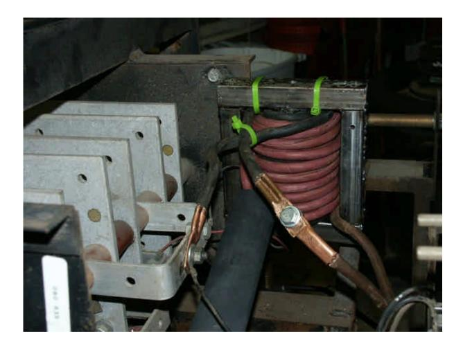
Above is one I made for my Miller. It is a 5" piece of 1.5" cast iron pipe wrapped in a steel frame. The wire is about 25 turns of #4 wire. Solid wire would work better, but stranded worked fine.
