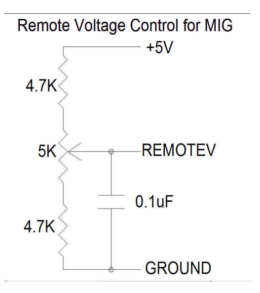
This will give a voltage range from 16.6 to 34.2 volts. If you do not plan on welding more than 100A or so, the upper resistor can be 10k. That will give about 16-25V out and an even finer control.
