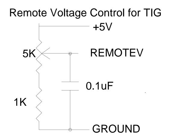
The potentiometer is the one in the footpedal. Use the current control to set the maximum current desired (full pedal setting.) Set the control board switches for remote contactor and voltage control.
