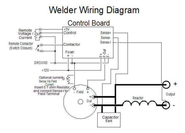
The above picture was for the large board. The simplified board has the Sense-, Power - and F-connections all tied to ground.
